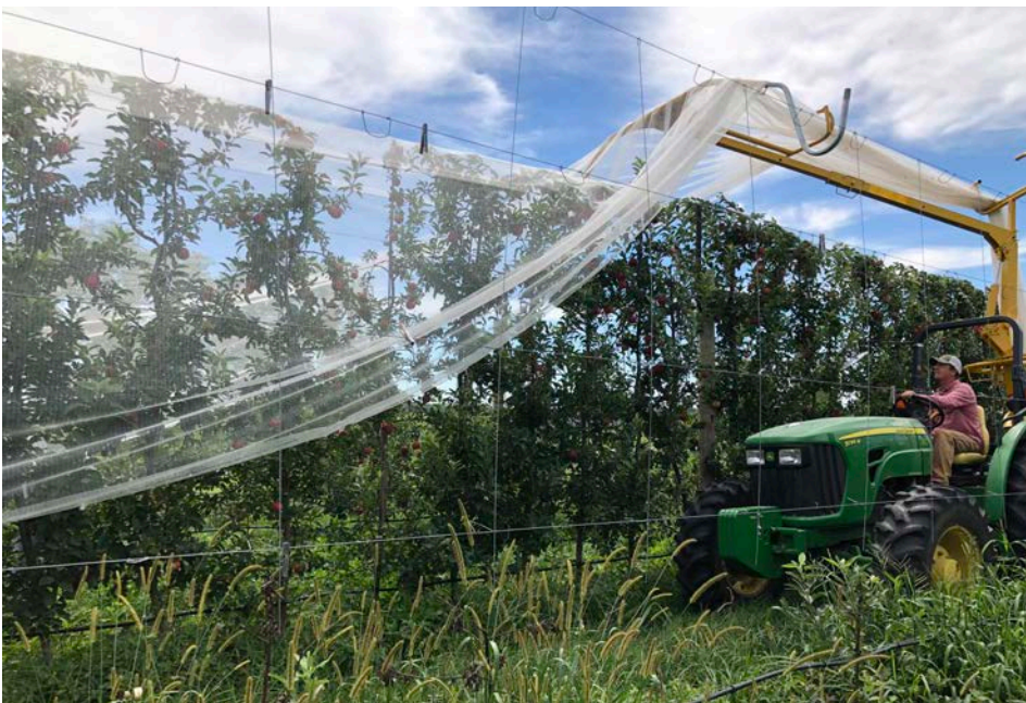
Removing the drape netting for apple harvest at South Baldwin Farm with the hydraulic mast applicator.
